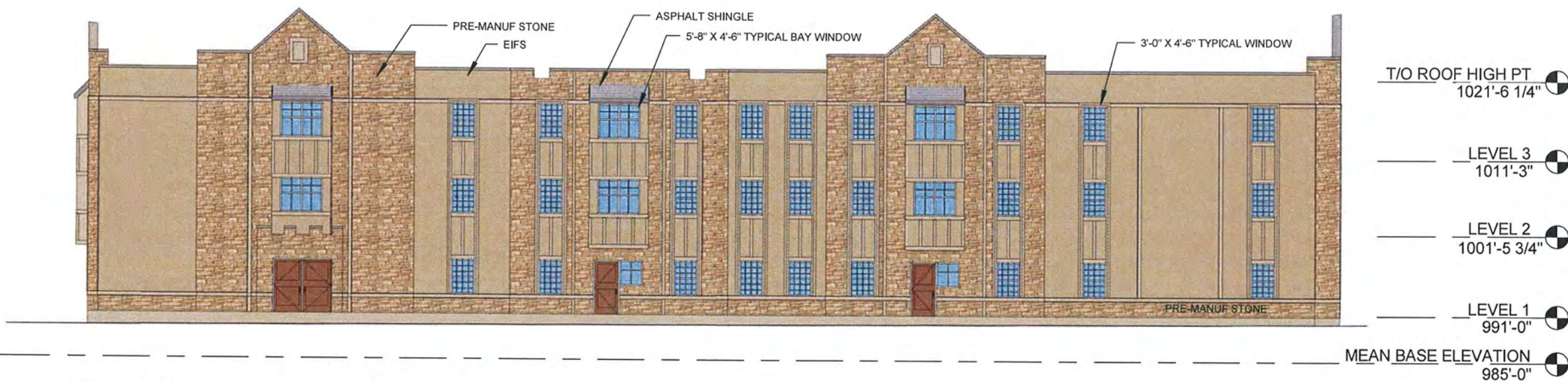
2 EAST ELEVATION - BRADFORD ST 400 1/16" = 1'-0"
