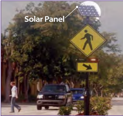
Figure 1: Activated, solar-powered RRFB on a center island at an unsignalized intersection—beacons flash using an irregular flash pattern that is similar to emergency flashers on police vehicles
