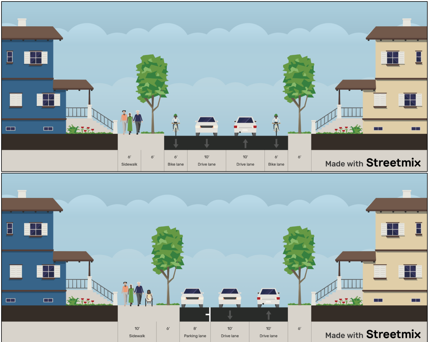
Figure 15: Design options for Camp Street with bike lanes (top) or with a multi-use sidepath (bottom)
