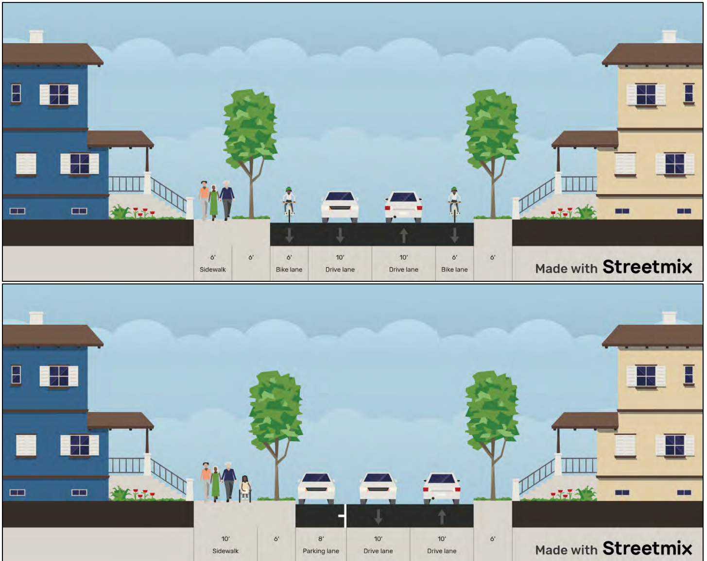
Figure 31: Design options for Camp Street with bike lanes (top) or with a multi-use sidepath (bottom)
