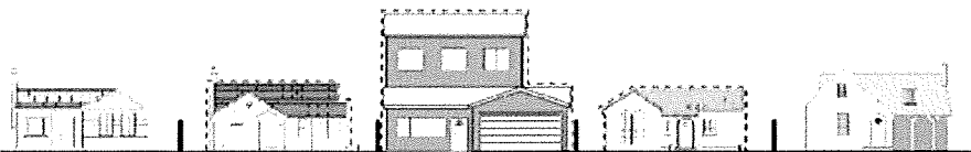
Figure 5. Middle building profile area is significantly larger than adjacent building profiles.
