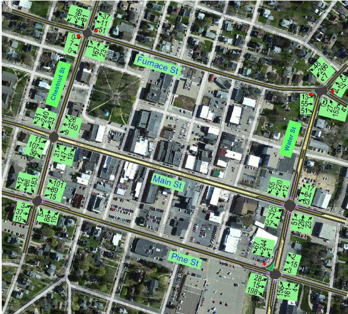
Figure 3.2: Downtown Platteville Street Network with the Addition of Traffic Signals at Main Street and Water Street With Morning Peak Hour Turning Movements
